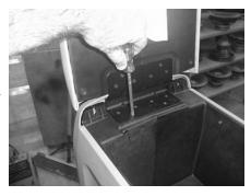
**STEP 6:** With a screwdriver, remove the six screws that secure the console lid.
